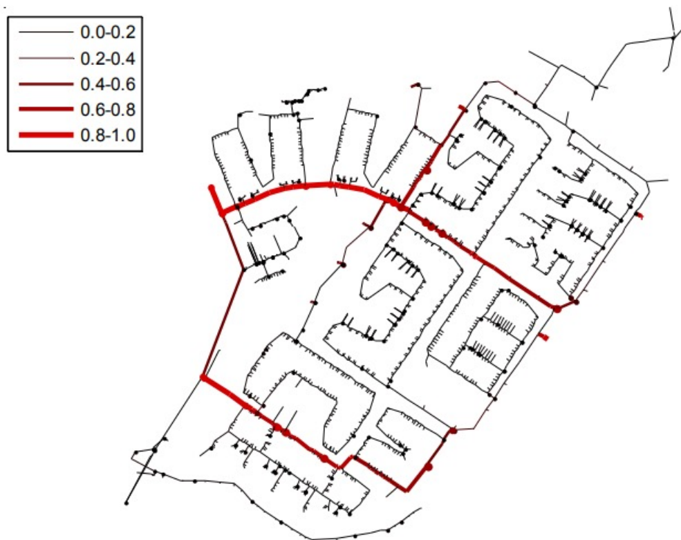
Figure 8-7. Percentage of time that pipe flow is turbulent pipes (0.01 h time step).
