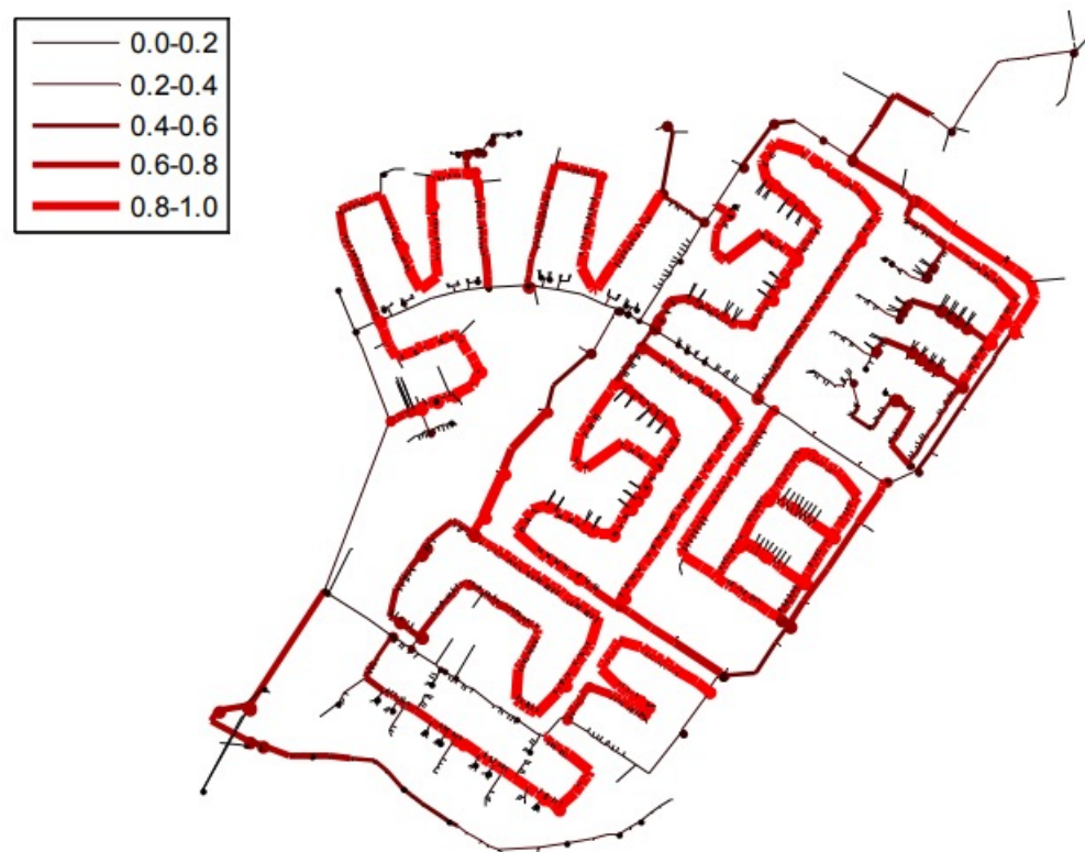
Figure 8-6. Percentage of time that pipe flow is laminar pipes (0.01 h time step). Re < 2000
