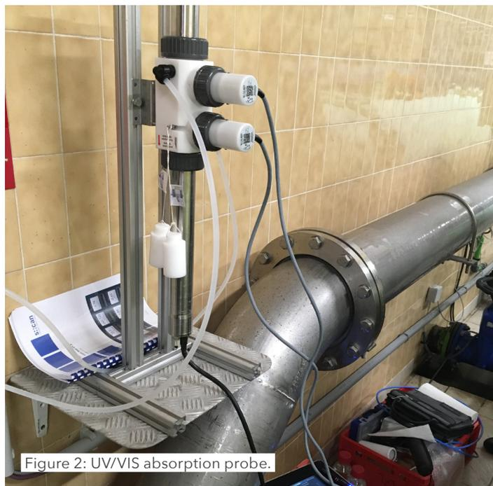
Figure 2: UV/VIS absorption probe.
