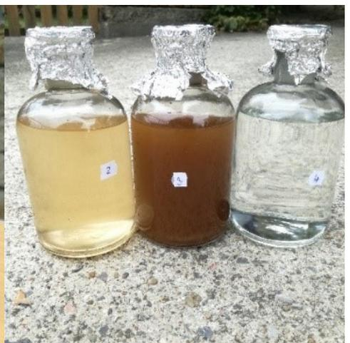
Fig. 3 Samples of the dirty water from the supply system during the flushing event
