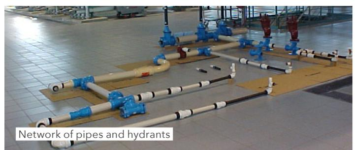
Dutch drinking water utilities have discussed at length with fire departments on required hydrant capacity. New build areas, with modern fire codes, and standard housing heights can do with 30 m<sup>3</sup>/h. High rise buildings and special buildings such as hospitals or shopping centres require special higher capacities.
