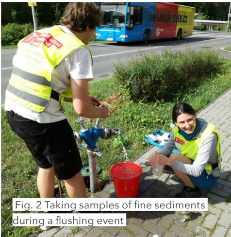
Fig. 2 Taking samples of fine sediments during a flushing event
